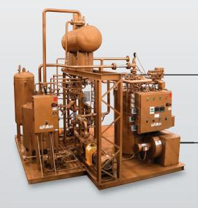
The skid system shown here included one FT-0240-C heater, a circulating pump, expansion tank and a temperature control unit (TCU). This system was designed to provide thermal fluid and hot water to several dryers for a wastewater application.
